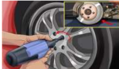
Figure2- 13 Unscrew the lug nuts and remove the wheel
