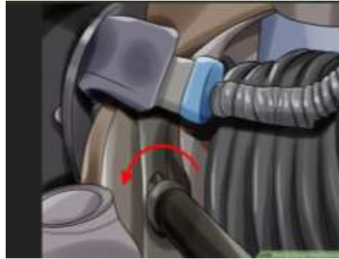
Figure2- 17 Unscrew the hub bolts and remove the old hub 9 Disassemble the hub assembly. To gain access to the bearings, you'll need to take apart the hub. You'll probably need to use a wrench (and/or a hammer) to remove the end of the hub and any anti-lock brake wheel that may be part of your hub. Then, you may need to use a specialized "puller" tool to remove the central bolt. The bearing assembly should come apart easily. See figure 2-18.
