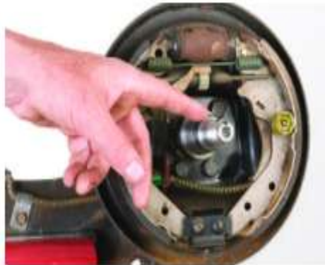
Figure2- 21 Clean and Inspect Hubs and Spindles
