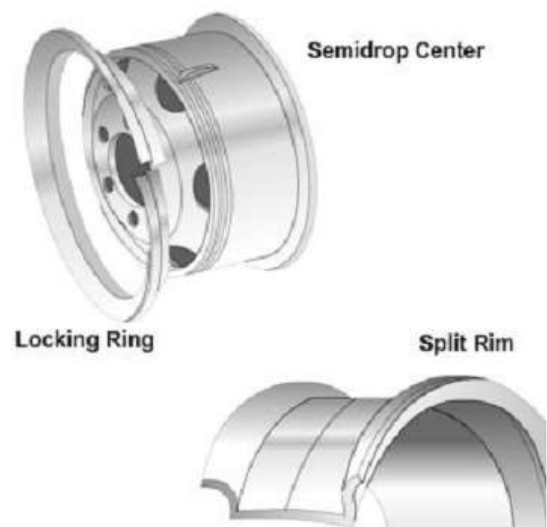
Figure2- 5 — Drop centre wheel
