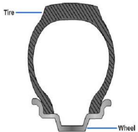
Figure2- 5 — Drop centre wheel
