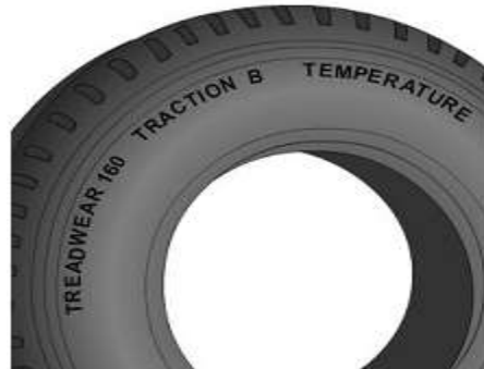
Figure2- 3 — Uniform tire quality grade system ratings on the sidewall of the tire
