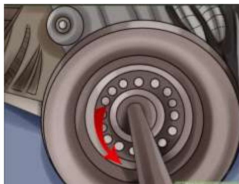
Figure2- 19 Remove races and cleans the knuckle
