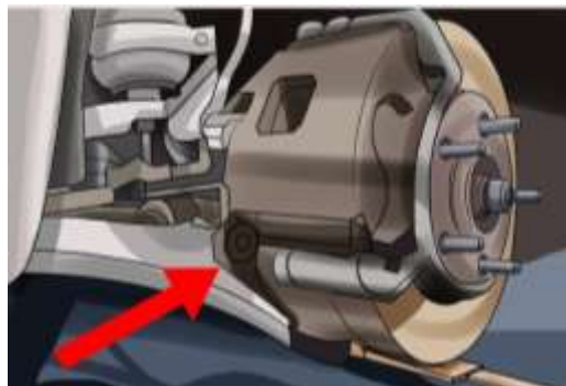
Figure2- 14 Remove the brake caliper
