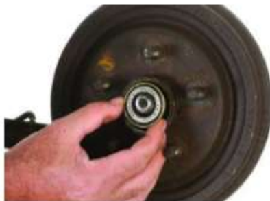
Figure2- 20 Wheel end disassembly
