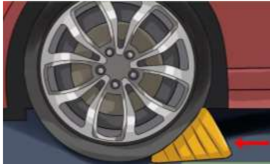
Figure2- 11 Use wheel chocks to secure wheels
