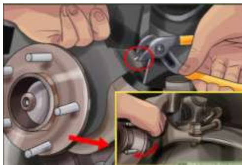
Figure2- 18 Disassemble the hub assembly 10. Remove races and clean the knuckle. Removing the bearing assembly's races usually means physically breaking them with a grinder or hammer and chisel. Because of this, you'll want to have replacement races ready. After removing the races, it's a good idea to clean the inside of the bearing assembly around the knuckle. See figure 2-19.
